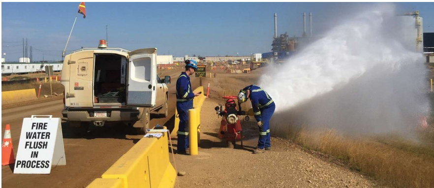
Hydrants Annual Flow testing and inspection
