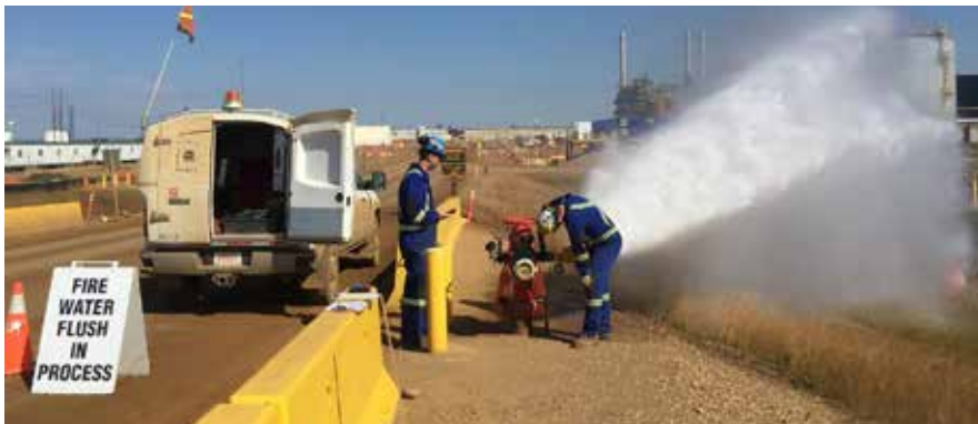
Hydrants Annual Flow testing and inspection
